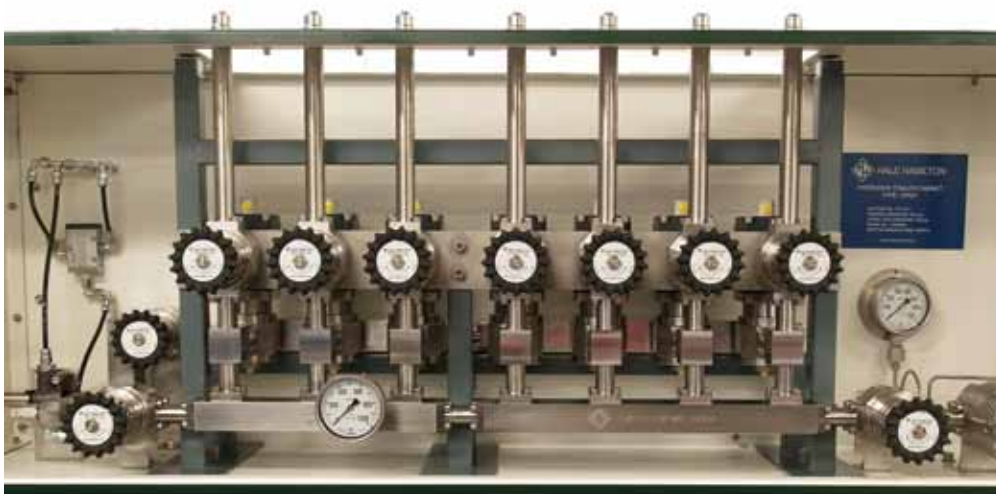
TPED certified manual and actuated stainless steel manifold for use with Hydrogen Trailers working at dual pressures of 200 and 500 bar with built in Dome loaded pressure regulator.
